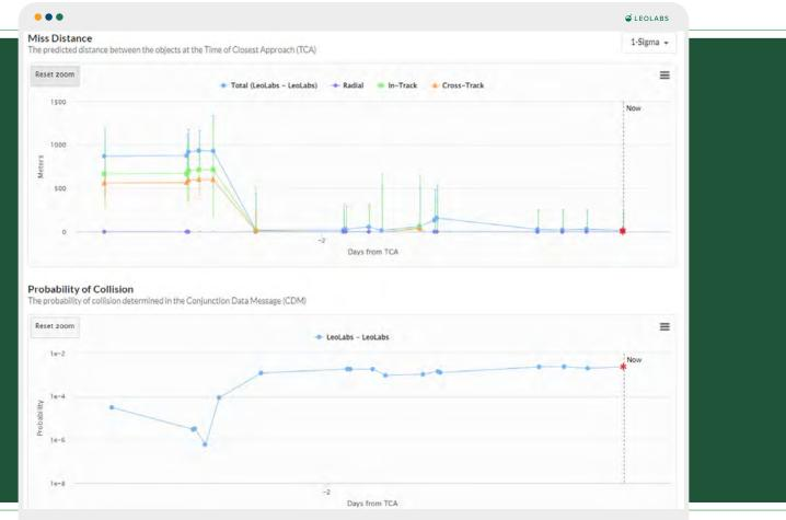
Figure 4 - Time history plots for miss distance and miss components, and probability of collision.
